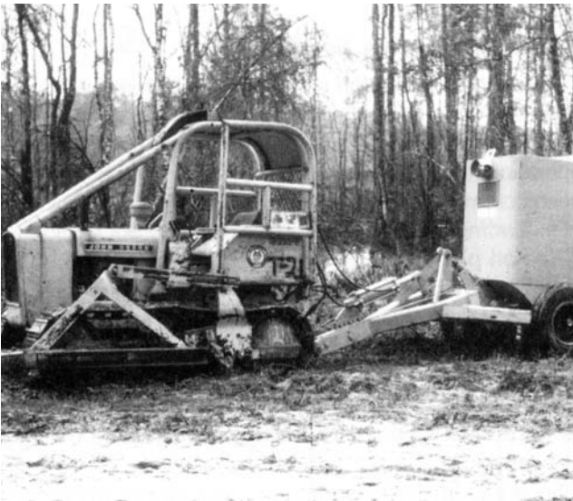
Figure 21. Heavy-duty mechanical planters are commonly used on large tracts and rough conditions.
